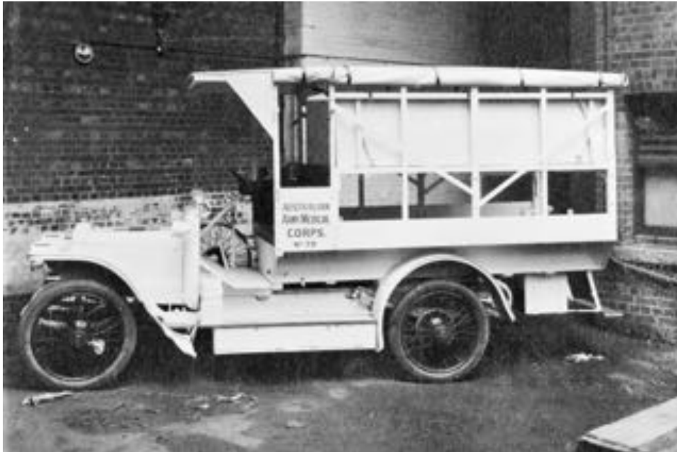
Above: A 1910 15 h.p. Daimler ambulance of the Australian Army Medical Corps. It is most likely the body was built in Australia. [Australian War Memorial PO2869.003]
