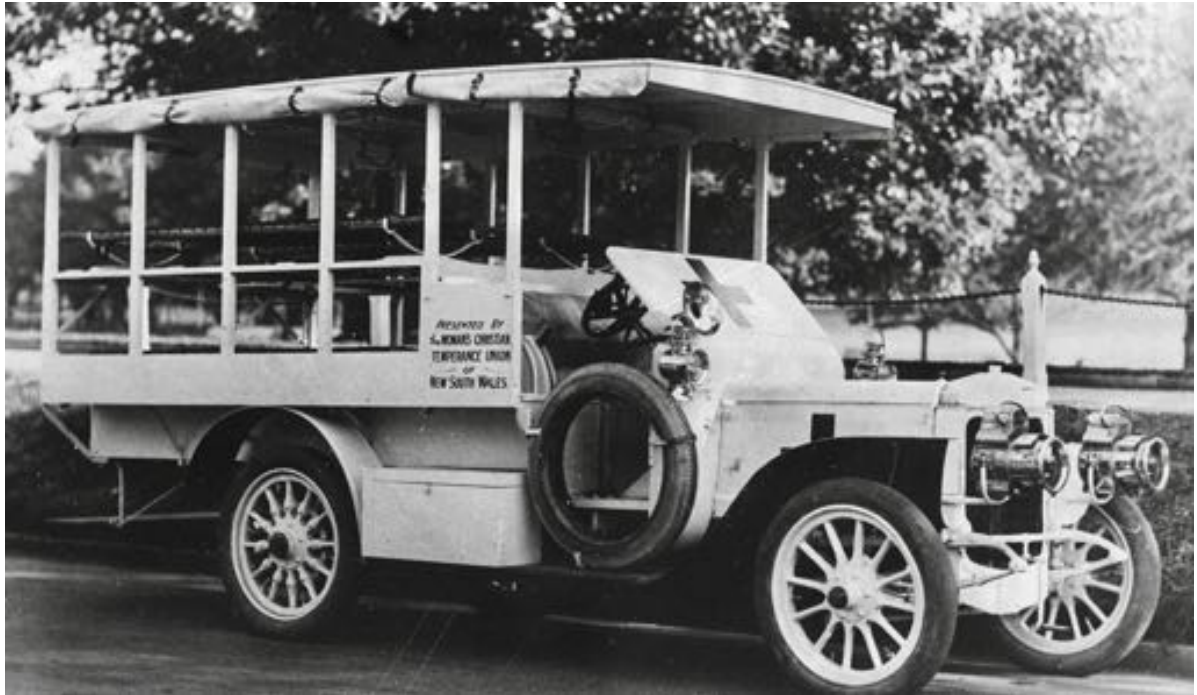
Above: An Australian body was built for this Daimler ambulance presented by the Woman's Christian Temperance Union of New South Wales. The motor body builder is not identified but was probably a firm in Sydney where the photograph was taken. The construction is the same as an ambulance body built by the Adelaide firm of Duncan & Fraser. It is likely both were constructed to the requirements specified by the military authorities. This image is from the State Library of South Australia [B56727] but appears to be reproduced from a photograph by Crown Studios, Sydney, held in the Sydney Powerhouse Collection of the Museum of Applied Arts & Sciences, see below.
