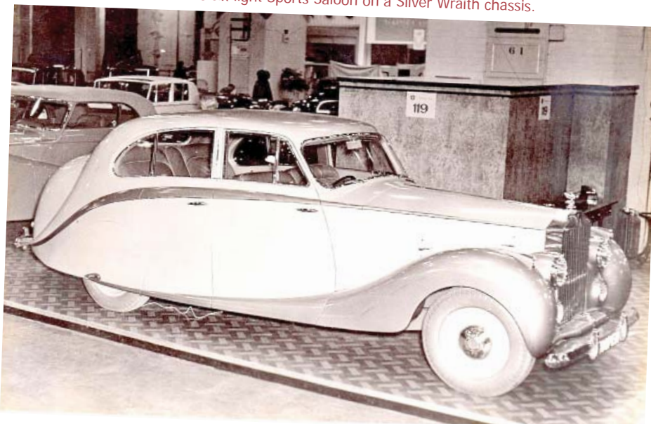
below: Hooper produced this six-light Sports Saloon on a Silver Wraith chassis.
