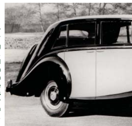
right: Hooper "Teviot III" Touring Limousine, all metal construction of aluminium alloy. The 1950 Earls Court Motor Show car, a Silver Wraith, WHD91.
