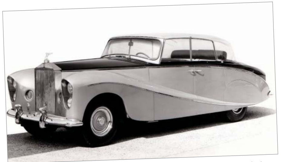
above: NS Gulbenkian Esq's Hooper Saloon with fixed transparent "Perspex" top. The top has "Perspex" ducts with refrigerated outlets and was fitted to 1956 Silver Wraith, LELW74.
