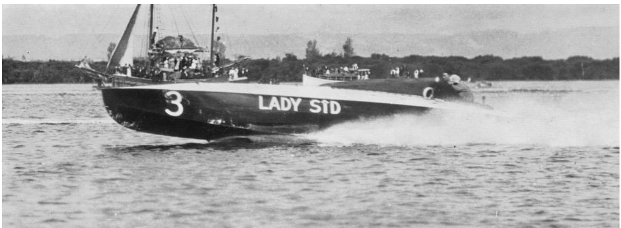
Below: Napier Birks was the mechanic when his daughter, Edith Napier Birks (1900-1975), was the pilot in 'Lady Sid'. Pictured here during 'The Griffith Australian Championship Cup' in 1924, 'Lady Sid' was a 33 foot single-step hydroplane fitted with a V-type 12 cylinder Thornycroft engine developing 375 h.p. Edith and Napier finished second in the race. [State Library of South Australia.]
