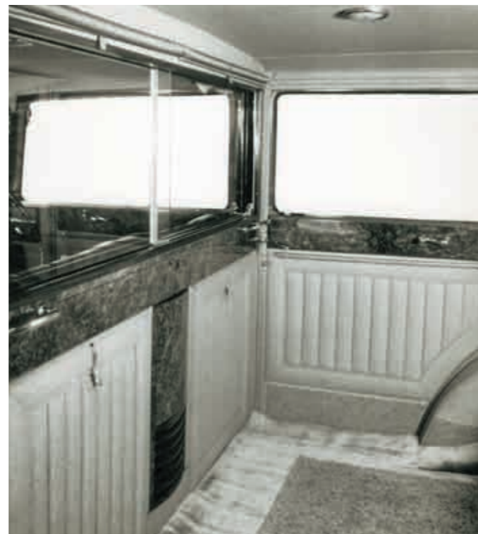
Below: 1. The interior of a new standard Hooper limousine, chassis number 3CM79. Beige cloth to the doors and the front of the disappearing occasionals, standard colour headlining, walnut woodwork, and a mohair floor mat. Note the sliding division window and the silk division roller blinds.
