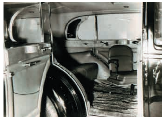
Below: 26. This is the interior of the first of three cars used by Rolls-Royce for display at the 1939 New York World's Fair, a Hooper limousine de ville on chassis 3DL156. Comment was made about the unusual rear quarter window blinds with panels of Purdah glass. Note also the swivelling armchair occasional seats, the electric division button, cigar lighter and radio controls on the elbows just inside the door and, just shown, the rear sunshine roof. The car was in black with fawn cloth to the rear compartment (and fawn leather to the front) and straight grain walnut woodwork.
