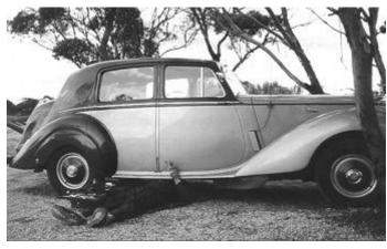
The petrol pumps are easily removed from under the chassis. To prevent emptying the fuel tank onto yourself, the siphon must be broken by removing the fuel filter cover.
