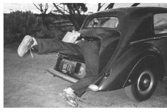
Access to the fuel filter is via two inspection plates at the rear of the boot secured to the boot and tyre compartment floors. A torch is needed.
