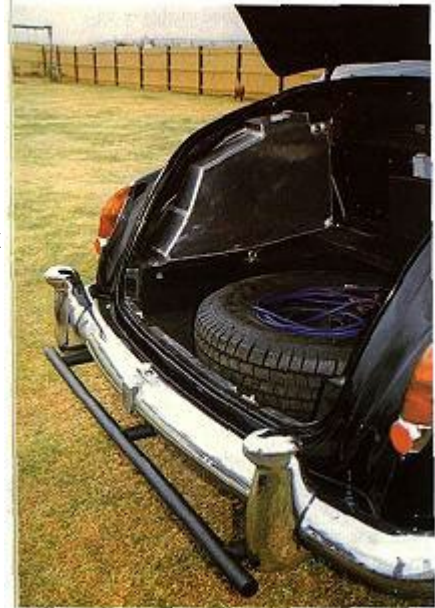
The standard 105 litre fuel tank is supplemented by an additional tank fitted into the left-hand side of the boot. Note the rear 'nudge-bar'.
