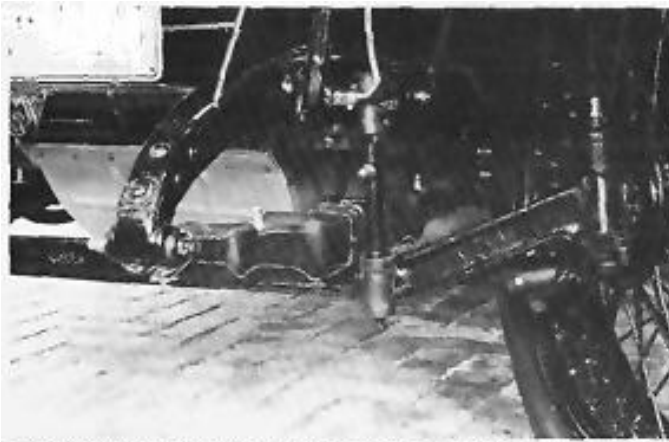
Front suspension showing Wefco gaiters, no brakes, a multitude of Enotts nipples, friction shock absorbers and the fitted undertray.
