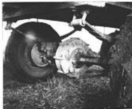
The rear axle of 1404 under the Riverina superphosphate cart in 1991. Note the modern steel disc wheels welded to the hubs.
