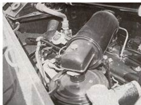
4BP3: the straight-eight engine. Note the oil-bath air cleaner, fitted for dusty countries. Silver Wraith and Silver Dawn owners will notice similarities.
