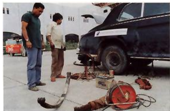
Kathmandu car-park. The broken, and previously welded, rear spring has been removed. New fabricated spring, still wrapped in hessian, in the foreground.
