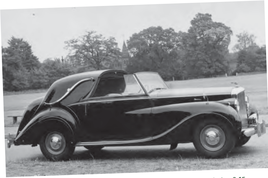
above: A James Young Bentley Mk VI 2 door Sedance Coupe, design C.15, 1947 -1950, 12 bodies built.
