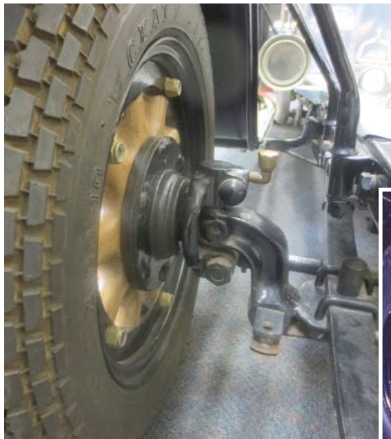
above: Detail of the wheel and front axle of the Silver Ghost model
