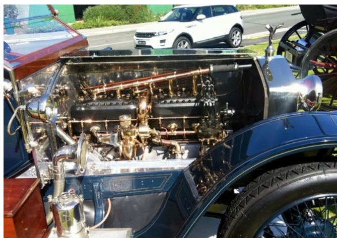
The big seven litre engine of the Silver Ghost. Nothing beats engine capacity. (Berg)
