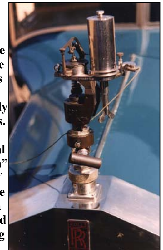
"I don't know what it does, but it does it magnificently". It is, in fact, a device for measuring the efficiency of steam engines.
