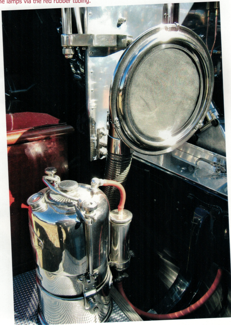
below: Before electric lighting on cars the most common form of lighting was by kerosene lamps or acetylene gas. The latter gave a brighter white light but it was more expensive and a little more troublesome. Here is a quality acetylene gas generator fitted to a Silver Ghost. The lower container is filled with carbide and the upper tank with water. An adjustable needle valve on top controls the amount of water allowed to drip onto the carbide below which generates the acetylene gas. The gas is passed through a filter then on to the lamps via the red rubber tubing.
