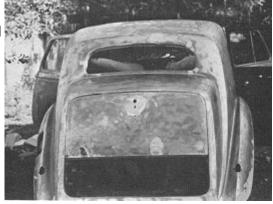
As Nick started to buff the car to get depth in the paint that he wanted - drama struck. The paint had not been put on thick enough and he was buffing through to the undercoat in patches.
