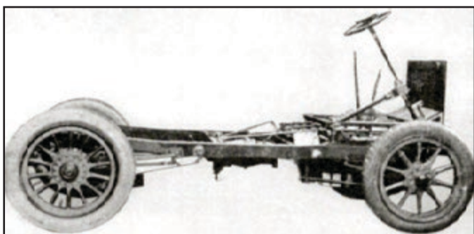
Off-side profile of a Legalimit Vee-8 reveals both the locations and the shallow depth of the engine above the chassis rails, together with the steering column bevel-case.
