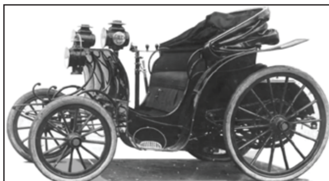
The chain driven 1898 Pre de Houf automobile with its engine mounted beneath the seat, and forward of the rear axle. (Image from the Houf Archive) is an earlier example of an under-floor-mounted engine, fitted to a chassis carrying classic horse-era styled coachwork. In this primitive attempt, the engine is mounted beneath the seat of the carriage.
