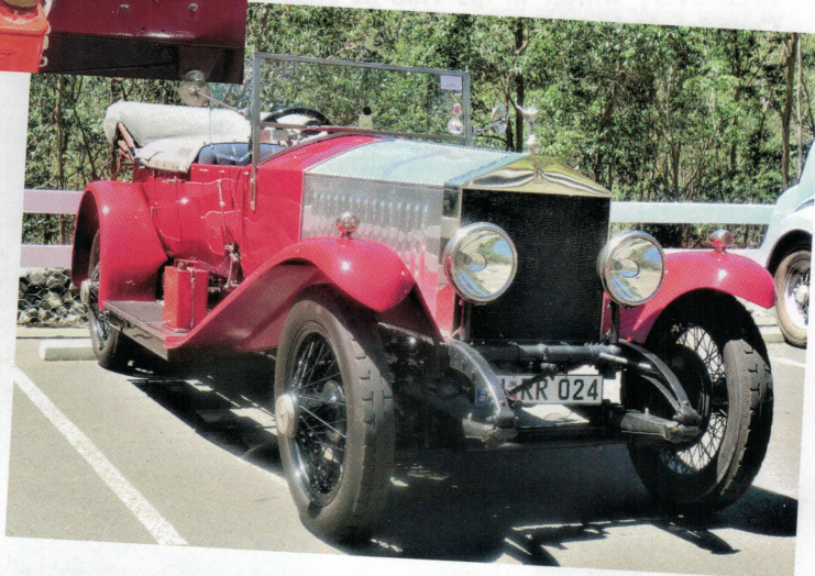
left & below: This long wheelbase 1924 Silver Ghost 123EM car came to Australia in 1924 with a Park Ward all-weather body. It has had many owners prior to being rebodied by Dubois of Melbourne in the 1990s. Narrow bodied tourers like this have difficulty accommodating the gear and hand-brake levers within the body and as in this case the brake lever was reshaped to fit outside the body. Since being rebodied this car has been owned by Rex Vincent of Sydney and he and his wife, Nora, have participated in many rallies in Australia, South Africa and New Zealand.
