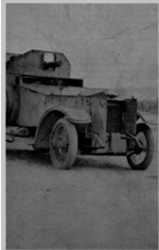
An armoured car at Mersa Matruh. Note bullet proof shutters to cover the radiator when under fire.
